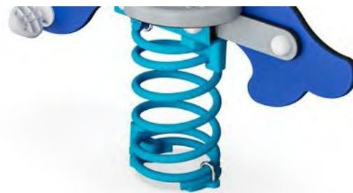
KOMPAN Springs are made of high quality spring steel according to EN10270. The springs are cleaned by phosphating before they are painted with an epoxy primer and a polyester powder coating as top finish. The springs are fixed by unique anti pinch fittings for maximum safety and long lifetime.
